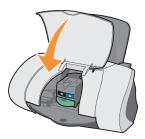
If the error message displays again, replace the black cartridge with a new black cartridge.
